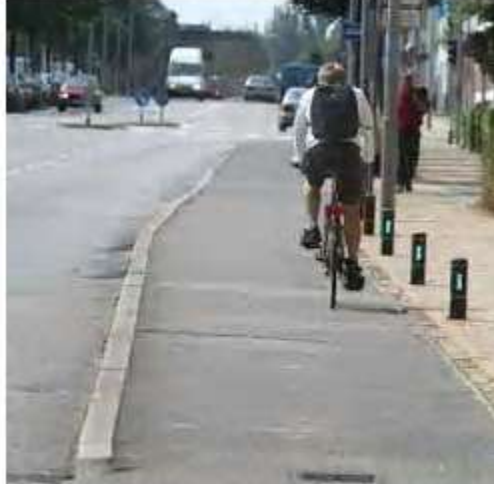
Green wave for cyclists in Odense, with bright green lights flashing on bollards just to the right of the lane to indicate correct cycling speed to achieve all green lights at intersections
