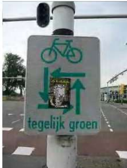
Traffic signal enabling four-way all-green crossing for cyclists in Groningen, avoiding all possible conflicts with turning cars
